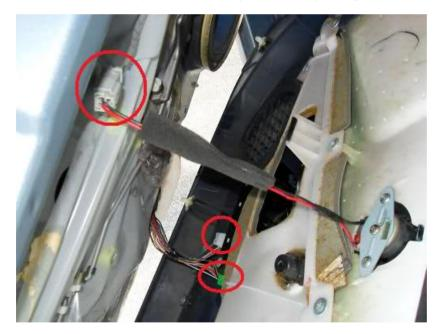
Okay now take your panel inside or wherever your going to be working on it. You will then need to remove the window switches. These are not held in by any screws or anything, look on the backside of the panel and you can see there is a long clip on the front of the module so it doesn't come out. Just push from the inside out on the back of the module and then just grap it from the outside, and pull it off
