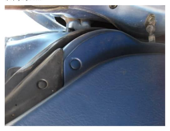
Next take out the two little plugs on the door handle, and there will be a phillips screw in each of these holes, remove both of those.
