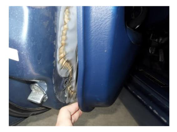
To remove the rest of the panel once its all popped loose, you will need to grab the panel and push upwards, toward the roof of the car. It should slide off. Dont yank the panel away or anything since your window controls and tweeters are plugged in still. On the driver side there are 3 connectors you need to un-clip, and on the passenger there are 2.
