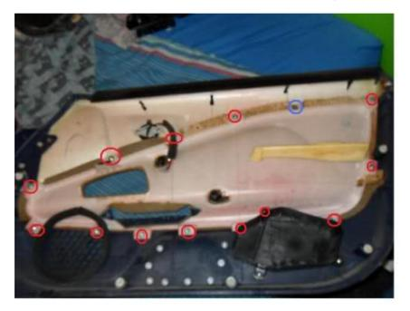
There is some foam like padding that goes around the speaker that is partly attached to the insert. If your new inserts have this still on it, just tear it where the end of the insert meets the panel, and install the new insert and it will make a whole. If your new insert does not have this on it, just carefully rip it where the insert meets the actual panel, and then remove it from just the insert. You can use adhesive to hold it onto your new inserts.
